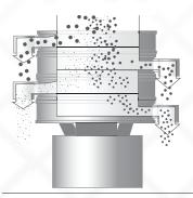
3 **Sizing:** Separation of particles into groups of like sizes. Accurate sizing of up to five product sizes can be achieved with one unit.
