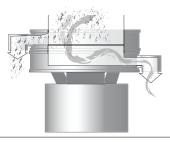
**De-watering:** Pre-filtering or de-watering for removal of solids from high throughput of liquids or slurries.
