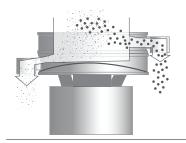
Scalping: Removal of a minimal amount of oversize product from volume throughput of good material.
