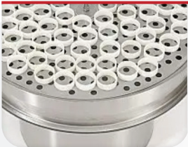
Slider Tray Recommended when blinding occurs due to wet, suspended particles.
